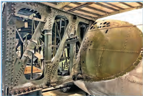
Disassembly of the Lacey Lady's Wing One
